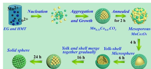
Scheme 1 Schematic illustration of the morphology evolution of the \text{MnCo}_2\text{O}_4 structure for different annealed time.
