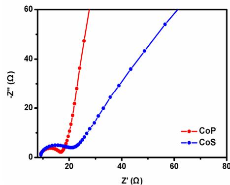
Fig. 4 Nyquist plots for CoS and CoP nanocatalysts.
