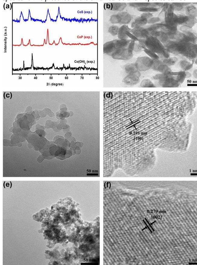
**Fig. 1** Structural characterizations of  $\beta$ -Co(OH)<sub>2</sub> nanoplate, CoS and CoP catalysts. (a) Powder XRD patterns of  $\beta$ -Co(OH)<sub>2</sub> nanoplate precursor and as-prepared CoP and CoS. (b) TEM image of  $\beta$ -Co(OH)<sub>2</sub> nanoplates. (c) TEM image of CoS. (d) HRTEM image of CoS. (e) TEM image of CoP. (f) HRTEM image of CoP.
