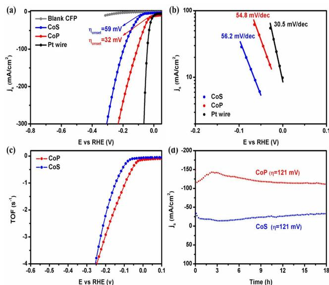
**Fig. 3** HER catalytic activity of the CoS and CoP nanocatalysts. (a) Polarization curves for Pt wire, CoS, CoP and blank carbon fiber paper (CFP) at a scan rate of  $5 \text{ mV/s}$ . (b) The corresponding Tafel plots for Pt wire, CoS and CoP. (c) The calculated turnover frequency curves for CoS and CoP nanocatalysts in our experiment. (d) Time-dependent current density.
