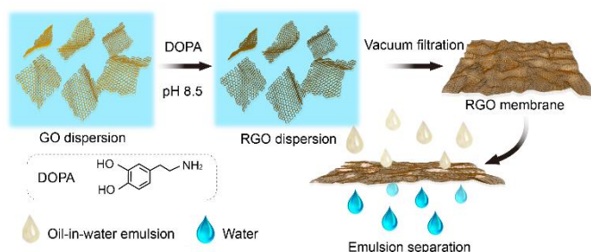
Fig. 1 Schematic illustration of preparing the free-standing RGO membranes and vacuum filtration process, and showing the separation capacity of oil-in-water emulsion.
