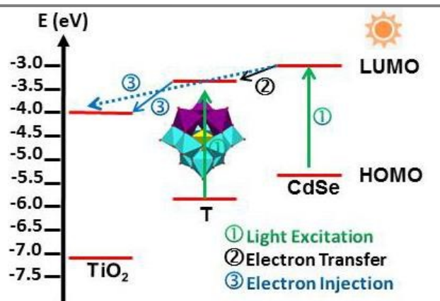
Fig. 7 The scheme of the charge separation processes for the TiO 2 electrode sensitized collaboratively by T and CdSe.
