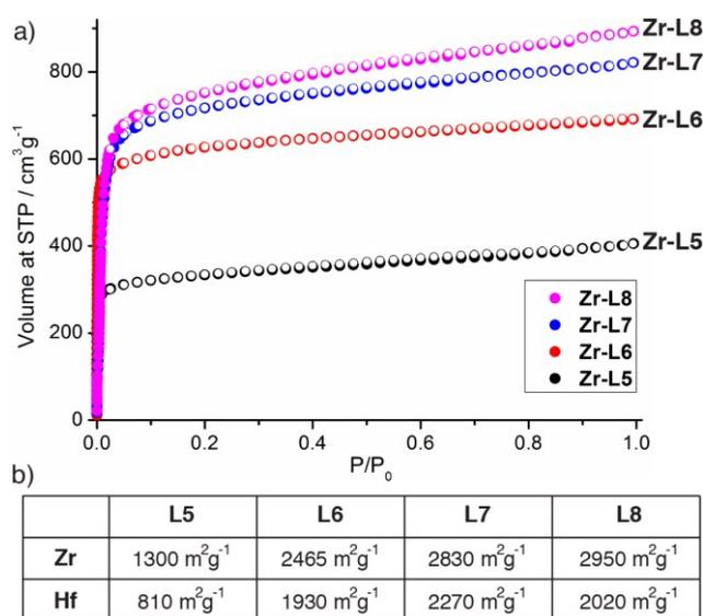
**Figure 6.** a) N<sub>2</sub> adsorption isotherms (77 K) for **Zr-L5**, **Zr-L6**, **Zr-L7** and **Zr-L8**. b) BET surface areas for all Zr and Hf MOFs, as derived from their N<sub>2</sub> adsorption isotherms.
