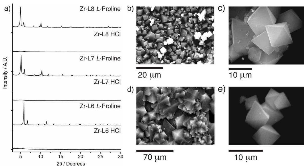
**Figure 2.** a) PXRD patterns showing the effects of incorporation of 5 equivalents of L-proline and one of HCl into solvothermal syntheses of Zr MOFs of **L6-L8** compared to addition of HCl alone. SEM images of the MOFs formed using this protocol: b) **Zr-L5**, c) **Zr-L6**, d) **Zr-L7**, e) **Zr-L8**.
