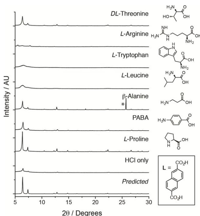
**Figure 1.** Stacked PXRD patterns of **Zr-L5** synthesised with different amino acid modulators (five equivalents), compared with **Zr-L5** synthesised with one equivalent of HCl only and the pattern predicted from the previously reported crystal structure.<sup>9b</sup> An unknown crystalline impurity, marked by an asterisk, was occasionally found in  $\beta$ -alanine modulated samples.
