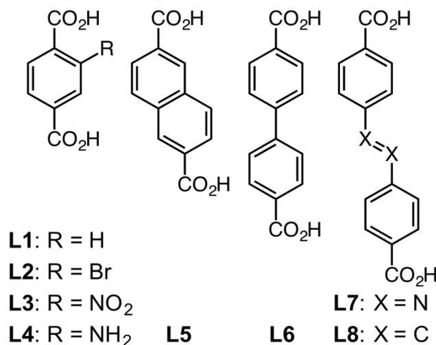
**Scheme 1.** Chemical structures of the dicarboxylate ligands, **L1-L8**, utilised in this study.
