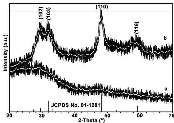
Fig. 1 XRD patterns of CuS QDs. (a) amorphous, (b) crystals.
