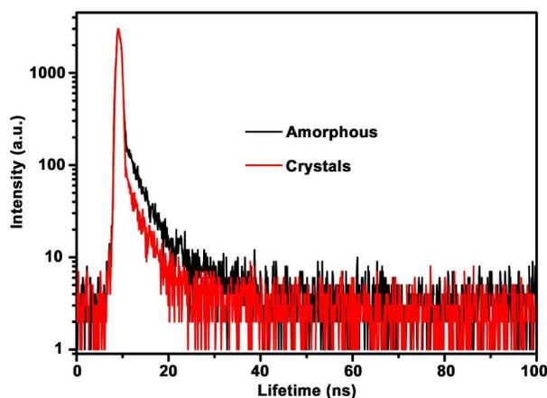
Fig. 5 Time-resolved photoluminescence of CuS QDs. (a) amorphous, (b) crystals.
