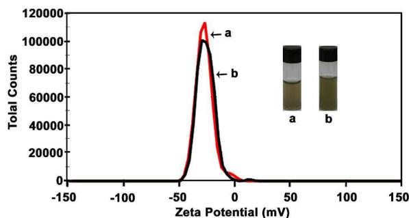
Fig. 3 The zeta potentials of CuS QDs. The red line is amorphous (a), the black line is crystals (b).
