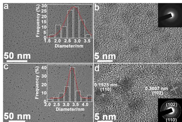
Fig. 2 HRTEM, SAED (inset) and particle sizes distribution (inset) of CuS QDs, (a) and (b) amorphous, (c) and (d) crystals.
