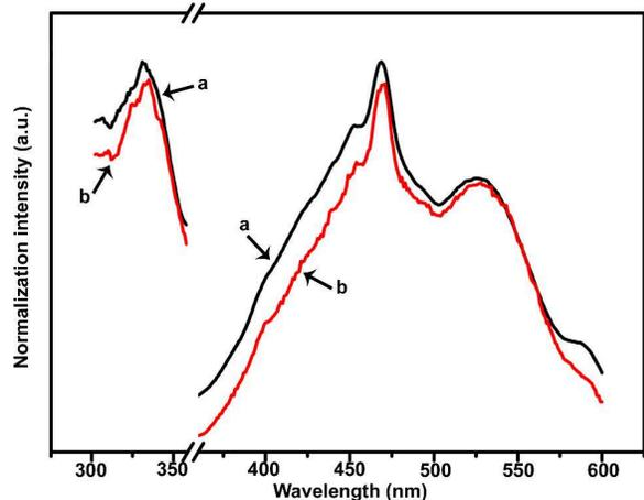
Fig. 4 PL spectra of CuS QDs, (a) amorphous, (b) crystals.
