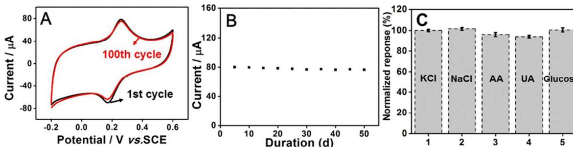
Fig. 8. The 1<sup>st</sup> and 100<sup>th</sup> CV curves (A) and the current for 50 days (B) of Pt/RGO/MnO<sub>2</sub> electrode in 0.1 M PBS (pH=7.0) solution containing 0.5 mM DA at scan rate of 50 mV s<sup>-1</sup>. (C) Results of interference study on the response of 100-fold KCl and NaCl, 10-fold AA, UA and glucose.
