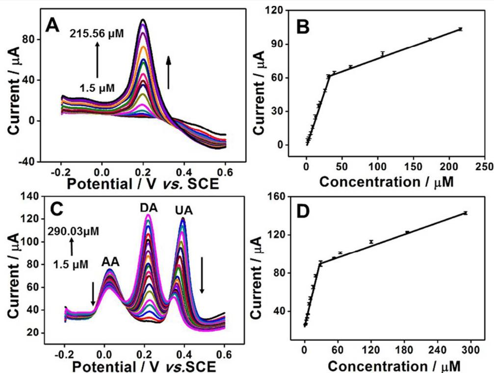
**Fig.7.** DPV curves of the Pt/RGO/MnO<sub>2</sub> electrode in 0.1 M PBS (pH=7.0) solution containing different concentrations of DA from 1.5-215.56 μM (A), 5 mM AA and 0.1 mM UA with different concentrations of DA from 1.5-290.03 μM (C). (B) and (D): Plots of oxidation currents versus the concentration of DA for corresponding spectra of (A) and (C), respectively.
