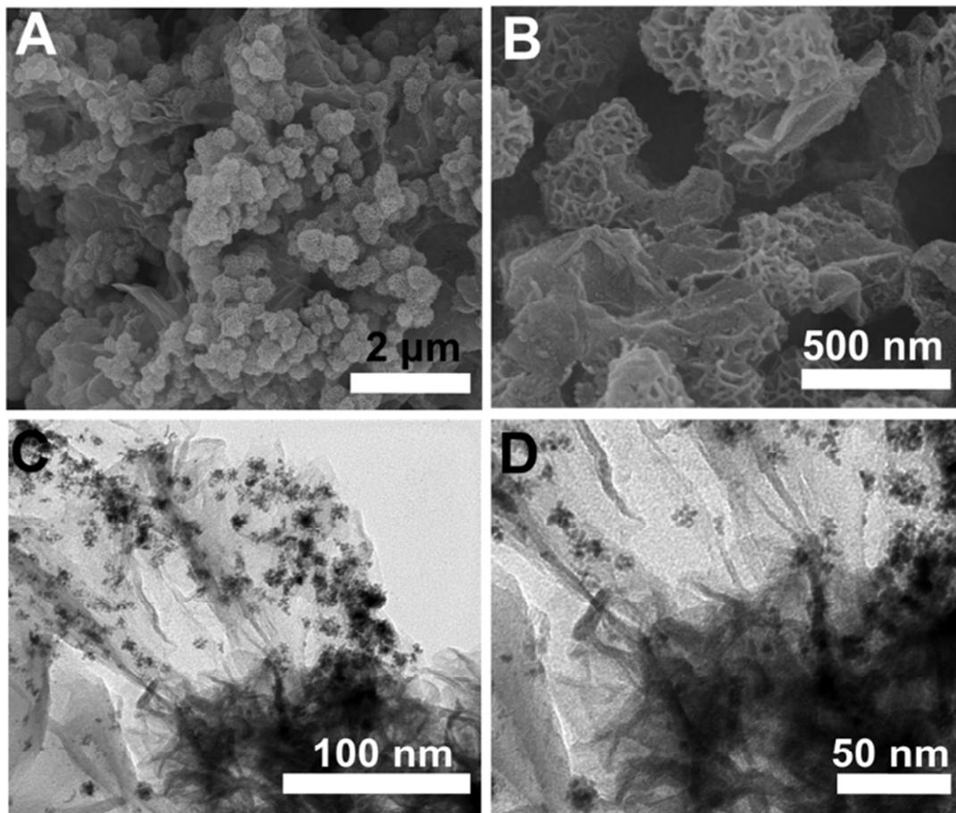
**Fig. 3.** SEM (A and B) and TEM (C and D) images of 3D Pt/RGO/MnO<sub>2</sub> nanostructures.
