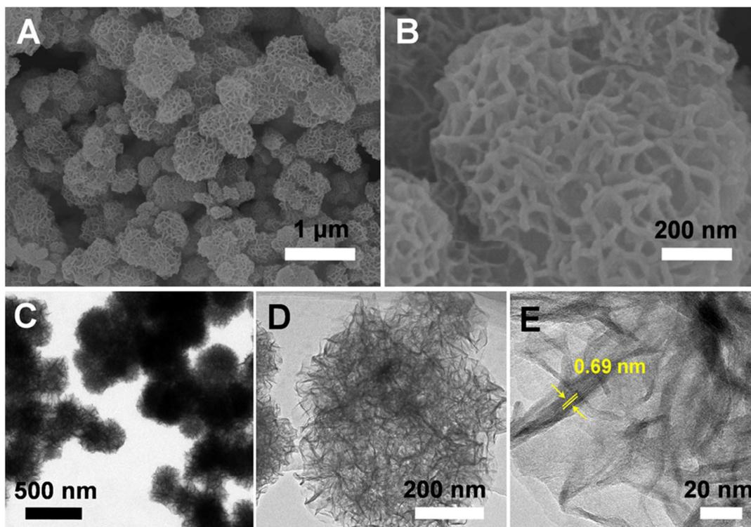
Fig. 2. SEM (A and B), TEM (C and D) and HRTEM (E) images of  $\text{MnO}_2$  nanoflowers.
