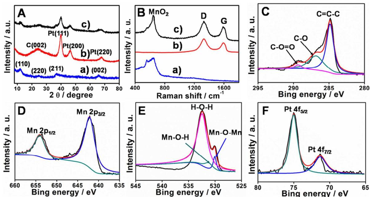
Fig. 4. XRD (A) and Raman spectra (B) of MnO<sub>2</sub> (a), Pt-RGO (b) and Pt/RGO/MnO<sub>2</sub> (c) nanocomposites. XPS spectra of C 1s (C), Mn 2p (D), O 1s (E) and Pt 4f (F) in the Pt/RGO/MnO<sub>2</sub> nanocomposites.
