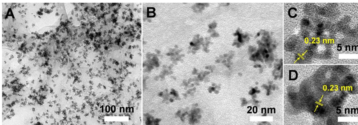
Fig. 1. TEM (A and B) and HRTEM (C and D) images of dendritic Pt/RGO nanostructures.
