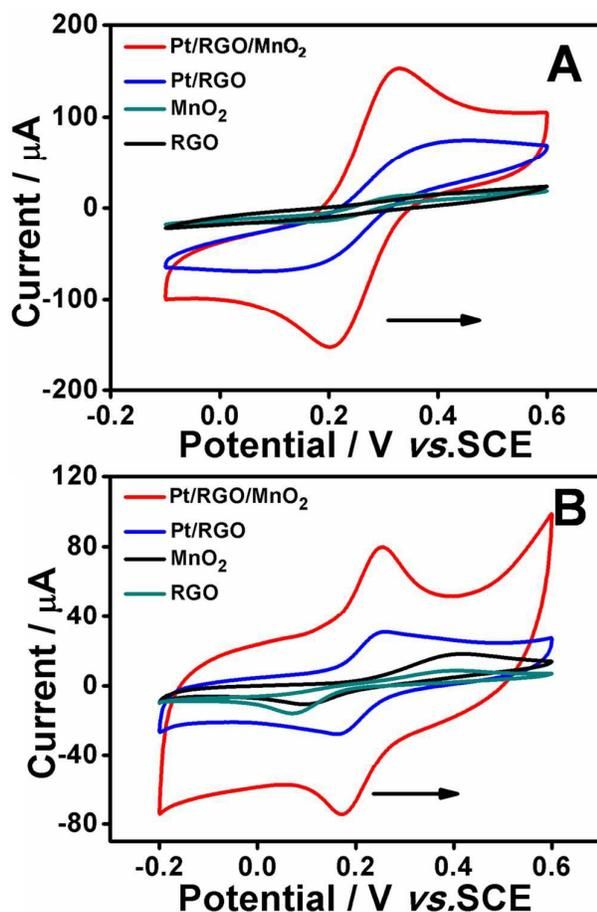
Fig. 5. CVs of Pt/RGO/MnO<sub>2</sub>, Pt/RGO, MnO<sub>2</sub>, RGO electrodes recorded in 10 mM Fe(CN)<sub>6</sub><sup>3-/4-</sup> + 0.1 M KCl solution (A), 0.1 M PBS (pH=7.0) containing 0.5 mM DA (B). Scan rate: 50 mV s<sup>-1</sup>.
