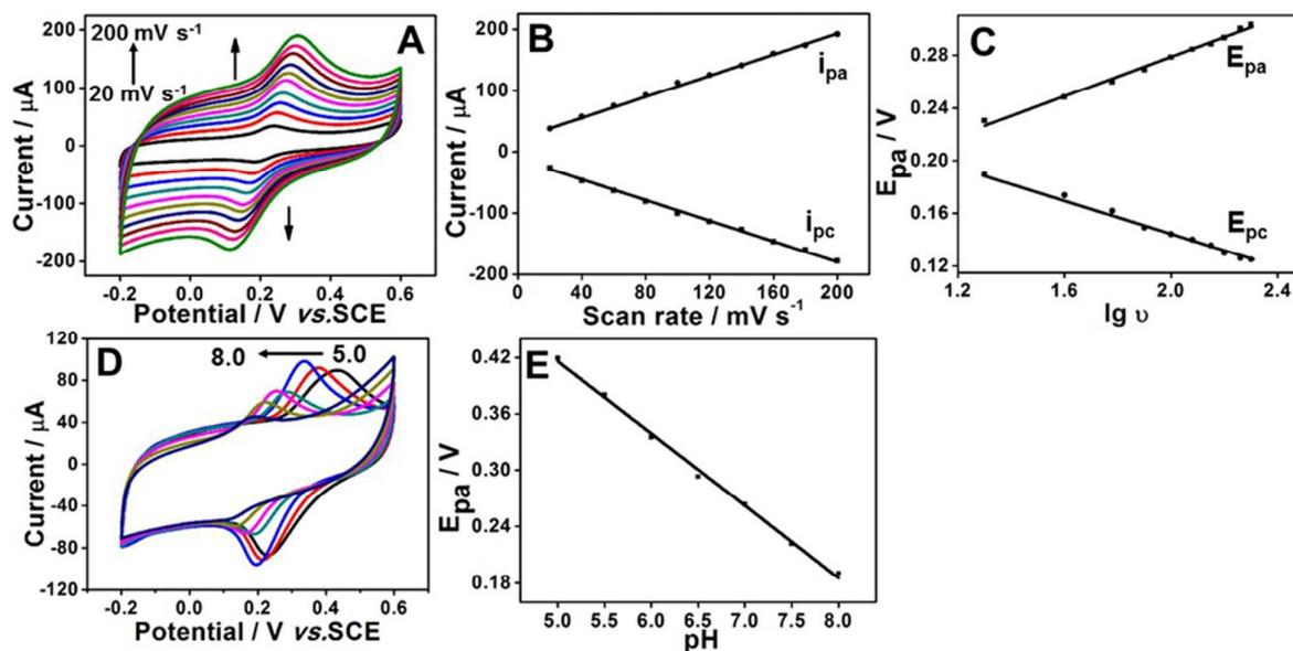
**Fig. 6.** CVs of the Pt/RGO/MnO<sub>2</sub> electrode in 0.1 M PBS (pH=7.0) solution containing 0.5 mM DA at scan rates from 20 to 200 mV s<sup>-1</sup> (A), 0.1 M PBS solutions containing 0.5 mM DA with the pH ranging from 5.0 to 8.0 (D). The plots of anodic and cathodic peak currents to the scan rates (B), anodic and cathodic peak potentials versus lg v (C), anodic peak potential against pH (E).
