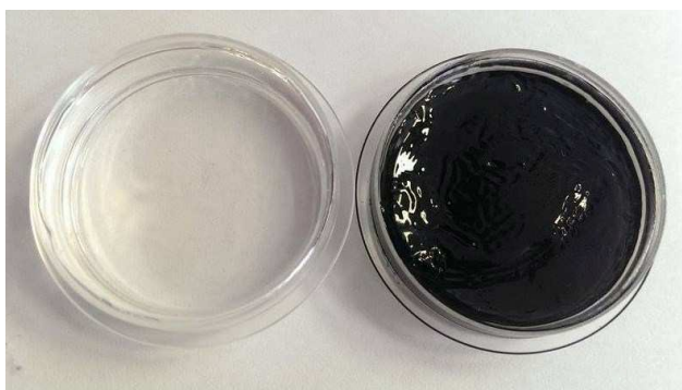
Figure 3. Photograph of the control hydrogel 8 (left) and of the photoantimicrobial hydrogel 7 (right) with 11 mg of 6 ( 10.30 \cdot 10^{-3} M stock solution in H 2 O) immobilized in it.
