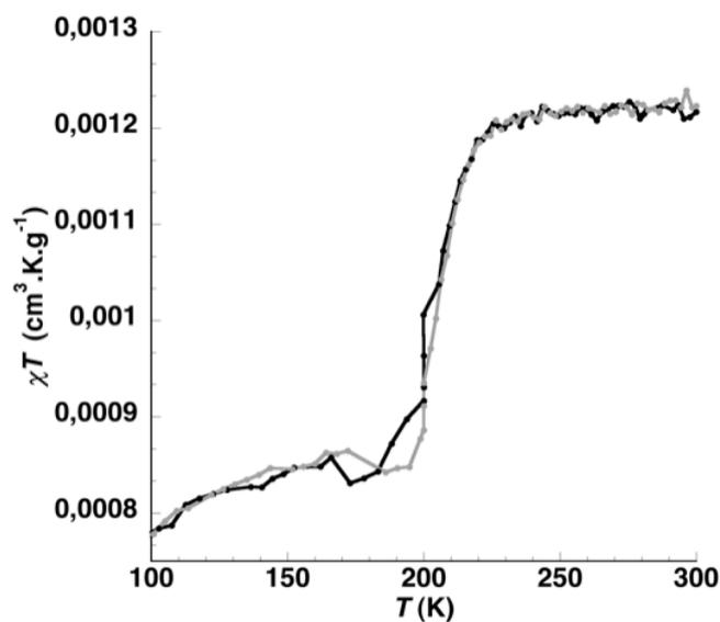
Figure 3. Product of the mass susceptibility by the temperature of a dried sample of the hybrid nanoparticles, recorded first while cooling from 300 K to 100 K (black) and then while heating from 100 K to 300 K (grey).
