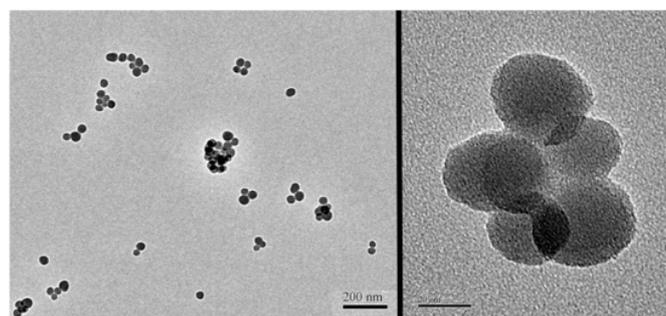
Figure 1. TEM images of the final hybrid silica nanoparticles. Left: scale bar is 200 nm, right: scale bar is 20 nm.
