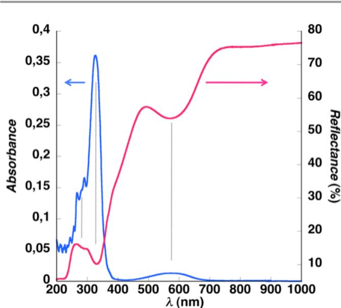
Figure 2. Absorbance (blue) spectrum of  $[\text{Fe}(\text{BIK})_3](\text{BF}_4)_2 \cdot 0.25\text{H}_2\text{O}$  ( $5 \cdot 10^{-5}\text{ M}$  in MeCN) and reflectance (pink) spectrum of the final hybrid nanoparticles (dried powder). The vertical dash lines are given as a guide for the eyes.
