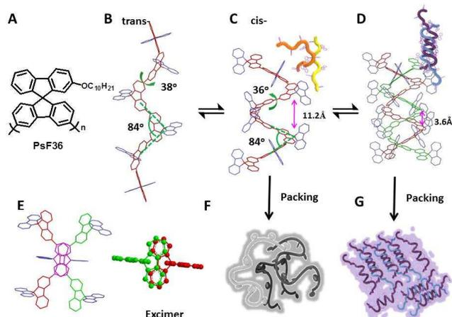
**Figure 1.** (A) Chemical structure of PsF36, (B) conformation of all *trans*-isomer, (C) conformation of all *cis*-isomer, (D) formation of double chain in PsF36 with *cis*-conformation, (E) the excimer formation in single chain packing, (F) the single chain packing with low fluorescence, and (G) the double chain packing with high pure violet emission.
