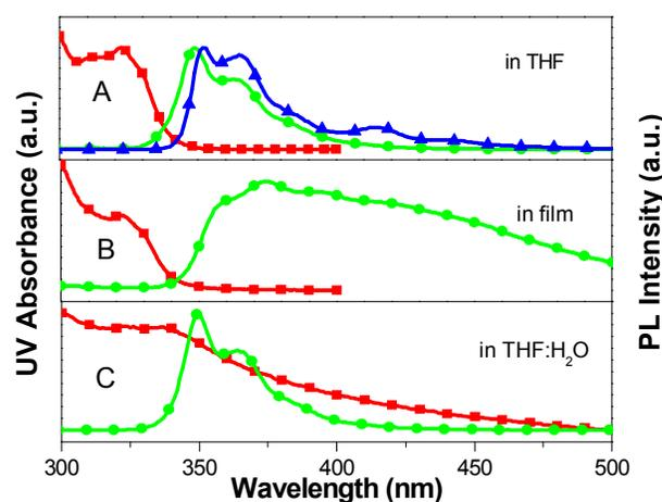
**Figure 2.** The absorption (square) and fluorescence (round and triangle) spectra of (A) PsF36 in THF,  $1.5 \times 10^{-5} \text{ M}$  (round),  $2.1 \times 10^{-3} \text{ M}$  (triangle); (B) PsF36 spin-coated film from THF solution; (C) PsF36 in THF:H<sub>2</sub>O mixed solution  $1.5 \times 10^{-5} \text{ M}$  (THF:H<sub>2</sub>O = 7:3).
