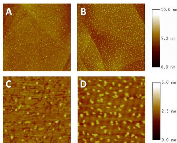
**Figure 5.** AFM height images of PsF36 spin-coated on HOPG plate substrates (A, C) from THF solution at a concentration of  $1 \times 10^{-5}$  M (by repeat unit); (B, D) from THF:H<sub>2</sub>O mixed solution, THF:H<sub>2</sub>O = 3:1 at concentration of  $1.5 \times 10^{-5}$  M. (A, B)  $3 \times 3 \mu\text{m}^2$ ; (C, D)  $1 \times 1 \mu\text{m}^2$ .
