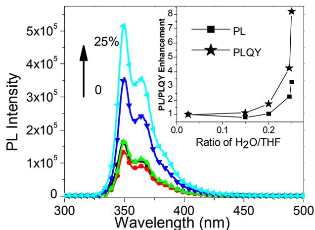
**Figure 3.** Fluorescence spectra of Psf36 in THF: $\text{H}_2\text{O}$  ( $7.5 \times 10^{-5}$  M) as a function of  $\text{H}_2\text{O}$  ratio. The spectra were measured at the excitation wavelength of 280 nm. The inset shows the evolution of relative PL intensity at 350 nm and apparent PLQY as a function of  $\text{H}_2\text{O}$  ratio, which is normalized by PL intensity and PLQY of Psf36 in THF ( $7.5 \times 10^{-5}$  M).
