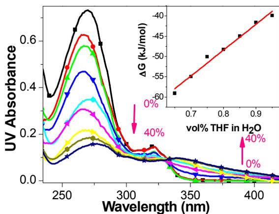
**Figure 4.** Detailed absorption spectra of PsF36 ( $1.5 \times 10^{-5}$  M) as a function of THF:H<sub>2</sub>O ratio. The inset shows Gibbs free energy change ( $\Delta G$ ) as a function of THF ratio.
