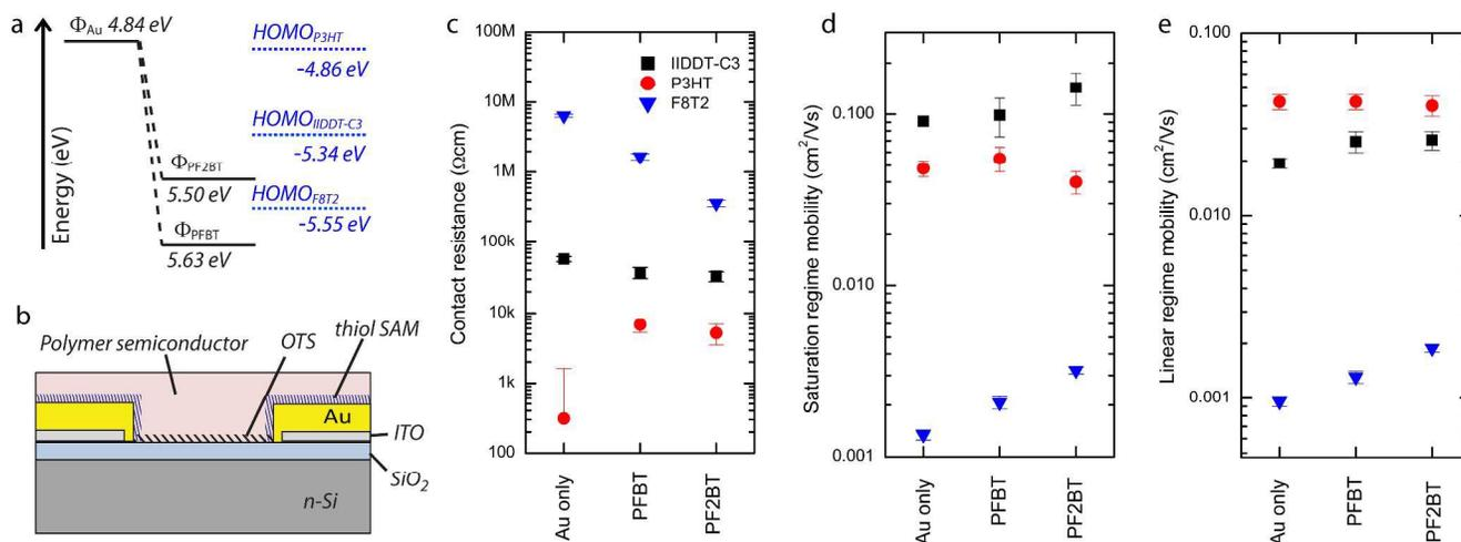
**Fig. 4** **a** Energy levels of the (modified) electrodes and the polymer semiconductors. **b** Schematic of the OFET structure. **c** Contact resistance, **d** saturation regime mobility and **e** linear regime mobility of the devices made with gold or SAM-modified electrodes and the three semiconducting polymers IIDDT-C3 (black squares), P3HT (red circles) and F8T2 (blue triangles).
