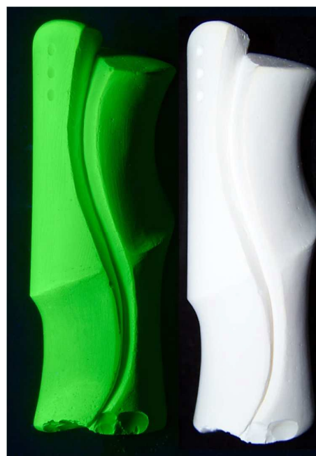
Figure 6. Photograph of sculpted piece of MSM-YAG:Tb composite with width/height dimension of 30/100 mm before (right) and after (left) 375 nm excitation.
