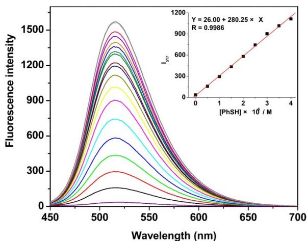
**Fig. 1** Emission spectra of **1** ( $5.0 \times 10^{-6}$  M,  $V_{\text{water}}:V_{\text{ethanol}} = 7:3$ ) upon titration of benzenethiol ethanol solution (0–10 equiv to **1**) with excitation at 380 nm. The linearity of peak intensity with respect to benzenethiol concentrations (inset).
