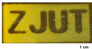
Figure 7 Liquid crystal physical gel for light scattering display at room temperature
