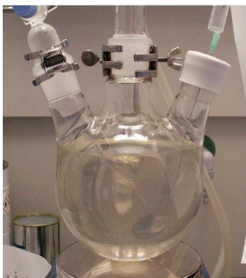
Figure 1. Typical precursor solution in the CO 2 method. The cannula in the upper right corner was used for introducing CO 2 .
