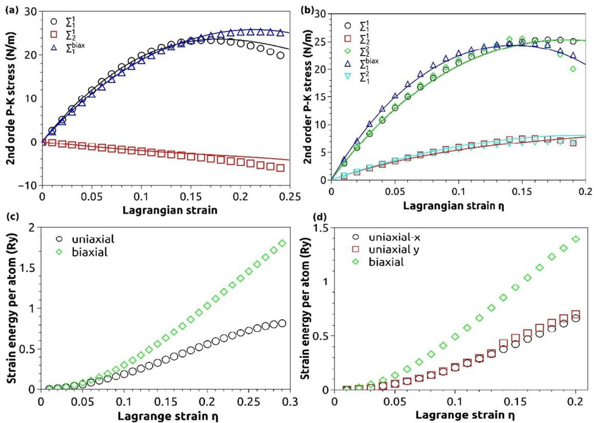
Figure 2. Stress strain curves for penta-graphene (a) and phagraphene (b). Energy–strain responses for penta-graphene (c) and phagraphene (d).
