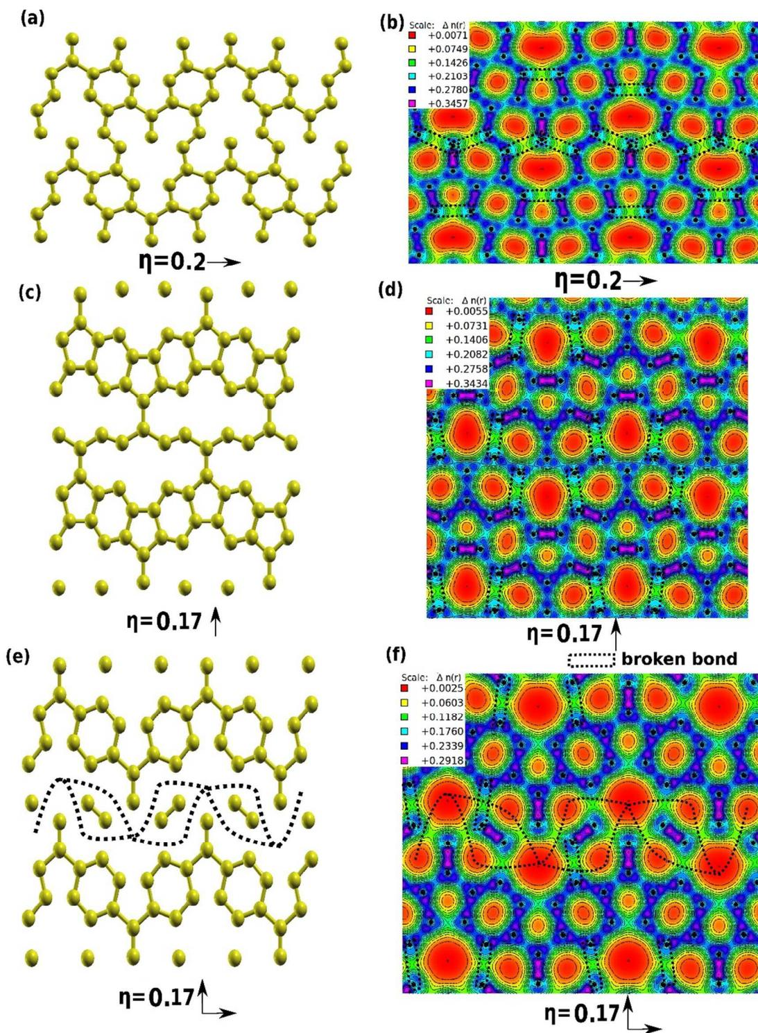
Figure 6. Charge density plot of phagraphene after (a)  $x$ -uniaxial tension for a strain of 0.2, (b)  $y$ -uniaxial tension for a strain of 0.17, and (c) biaxial tension for a strain of 0.17. The dashed lines show the fracture pathways. The broken bonds are emphasized by black rectangles. The “Scale” legend represents the relative density of electrons, the unit for electron density is  $1/\text{\AA}^2$ .
