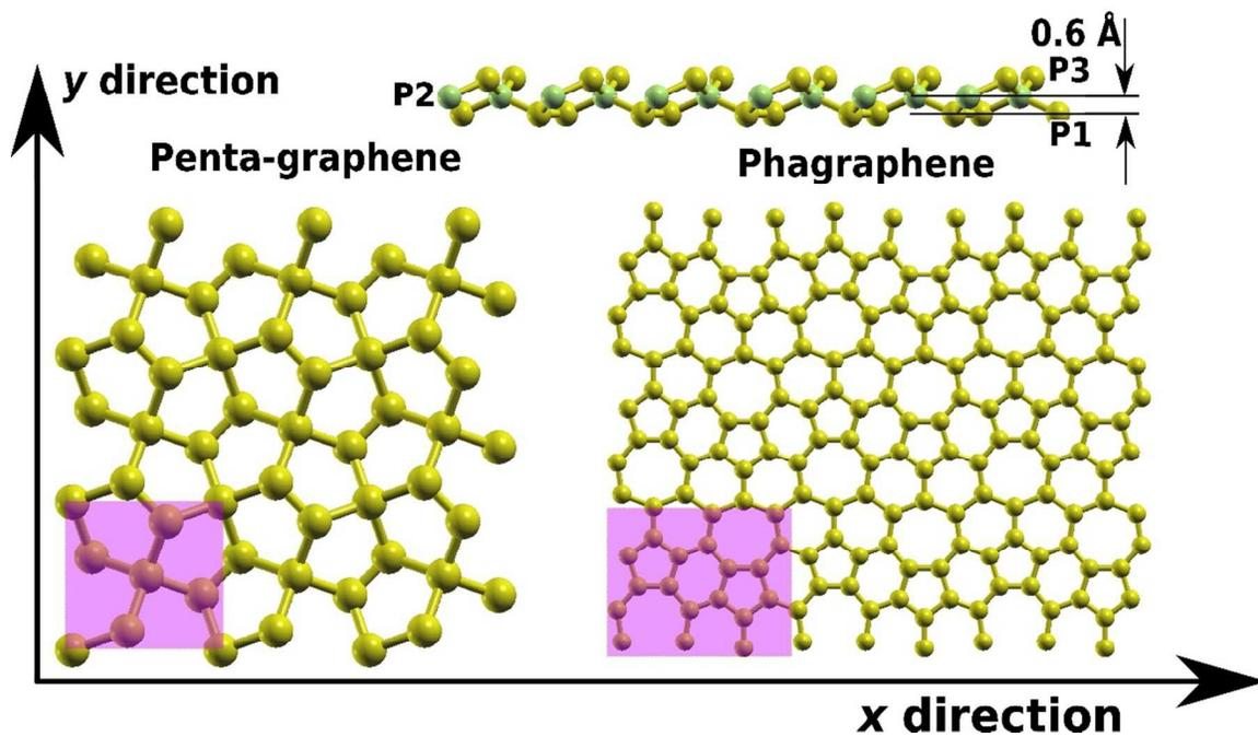
Figure 1. Schematics of the atomic structures for penta-graphene and phagraphene. Unit cells are shown in pink. Side views of penta-graphene are shown on the top of this figure with three planes of atom. The atoms in P2 plane are marked in green.
