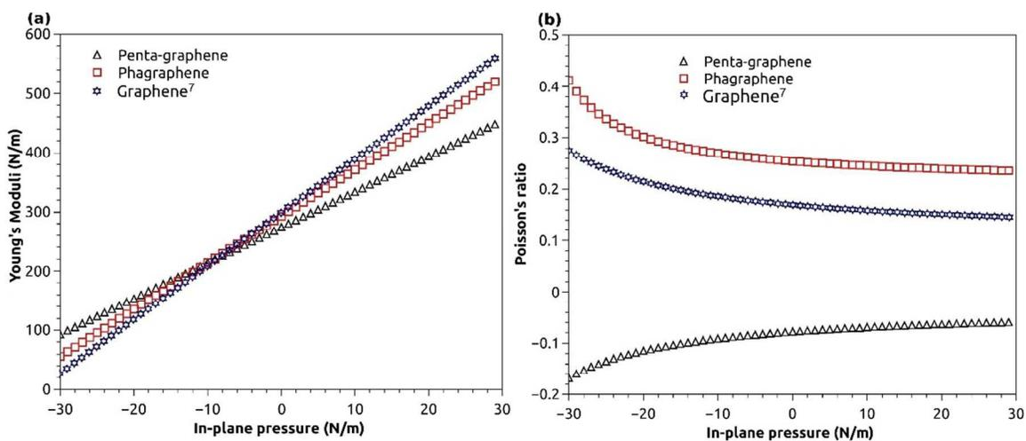
Figure 4. (a) Second-order elastic moduli (b) and Poisson's ratio as a function of the in-plane pressure for graphene, penta-graphene, and phagraphene.
