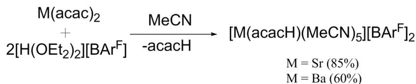
Scheme 2: Synthesis of  $[\text{M}(\text{acacH})(\text{MeCN})_5][\text{BAR}^{\text{F}}]_2$  ( $M = \text{Sr}$ ,  $\text{Ba}$ )
