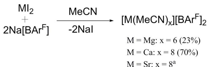
Scheme 1: Synthesis of  $[\text{M}(\text{MeCN})_x][\text{BAR}^{\text{F}}]_2$  ( $M = \text{Mg}$ ,  $\text{Ca}$ ,  $\text{Sr}$ )
