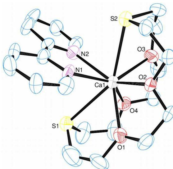
Figure 4. The cation of  $[\text{Ca}([\text{18}]aneO_4S_2)(\text{bipy})][\text{BAr}^F]_2$ . Ellipsoids are shown at the 50% probability level and the hydrogen atoms omitted for clarity. Selected bond lengths (Å) and angles (°): Ca–O1 = 2.497(6), Ca–O2 = 2.433(6), Ca–O3 = 2.514(6) Ca–O4 = 2.462(6), Ca–S1 = 2.943(4), Ca–S2 = 2.935(4), Ca–N1 = 2.461(7), Ca–N2 = 2.458(7); S1–Ca–S2 = 145.23(9), S1–Ca–O1 = 67.7(2), O1–Ca–O4 = 87.0(2).
