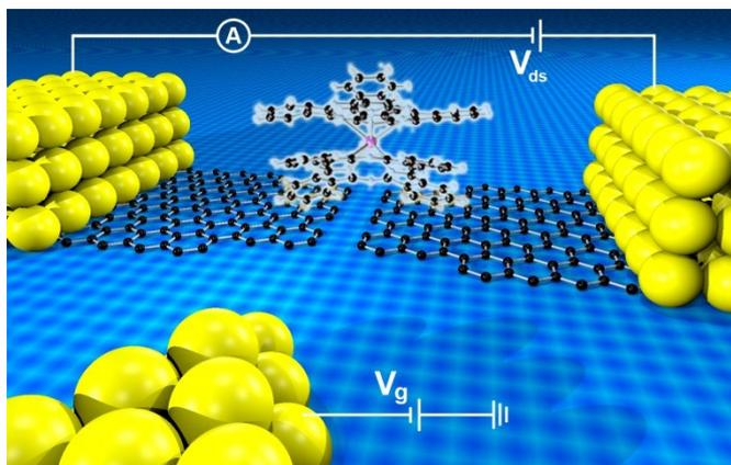
**Figure 1.** Artist's impression of the molecular device with graphene electrodes and a TbPc<sub>2</sub> single-ion magnet located in the junction. A lateral gate electrode approaches the nanogap. The measurement set-up is also displayed in the schematics.
