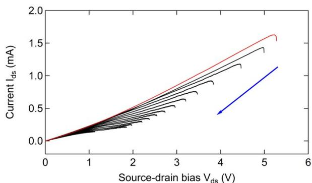
**Figure 2.** Set of I-V characteristics showing the evolution (see blue arrow) of the feedback-controlled EB process. A voltage ramp is applied across the device until its resistance increases by more than a predefined percentage. The process is iterated until the low-bias resistance reaches 100 k $\Omega$  – 4 M $\Omega$ .
