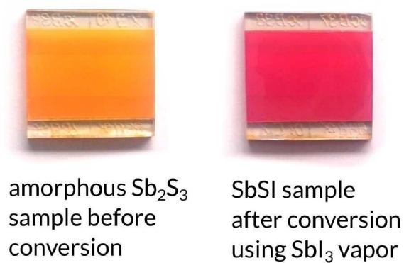
Fig. S1 Photograph of an amorphous \text{Sb}_2\text{S}_3 sample and a SbSI sample after conversion with \text{SbI}_3 and rinsing in ethanol.
