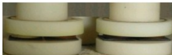
Figure 1. Samples of CROFER22 APU in contact with apatite pellets. Sets are kept under constant uniaxial pressure using alumina plates.
