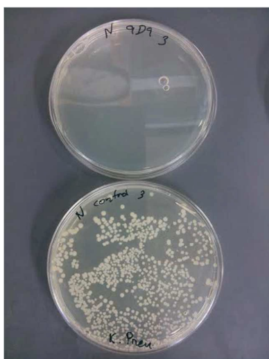
Figure 2: Photo of agar plates incubated with a solution of K. pneumoniae after being passed through an AgNP@Klig/PAM equipped filter plug (top), and a Klig/PAM equipped filter plug (bottom).
