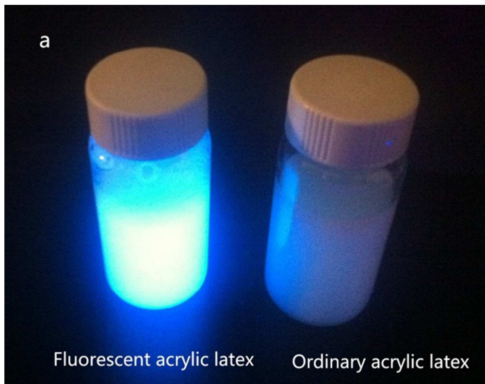
Fig.2 (a) Fluorescent acrylate emulsion and ordinary acrylate emulsion irradiated under UV light
