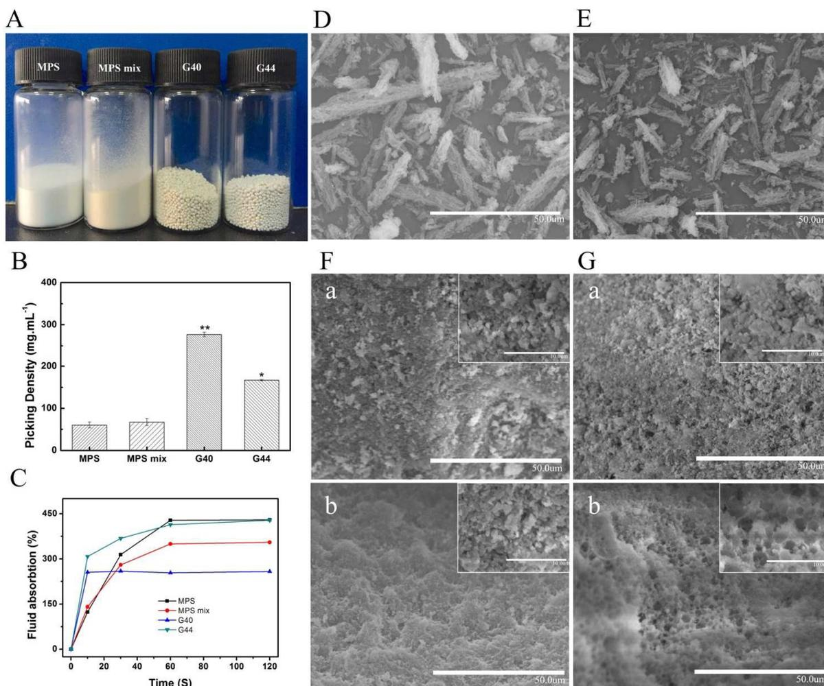
Fig. 1 A: photos of MPS, MPS mix, G40 and G44; B: packing density of samples; C: water absorbability of samples; D-G: SEM of MPS, MPS mix, G40 and G44 (a: outer surface, b: cross section); \* $p < 0.0008$ , \*\* $p < 0.0003$ : significantly different from control.
