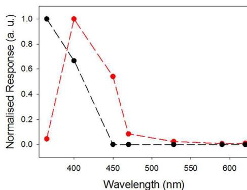
**Figure 8** Comparison of normalised photocurrent of xerogel-1,2 (red), and xerogel-1 (black data) at different wavelengths. The responses were measured at 4V from using a 2 electrode set up, see Fig. S8 and Fig. S9. Data at the different wavelengths were collected for the same samples at different wavelengths after allowing full recovery to baseline before a new measurement was carried out.
