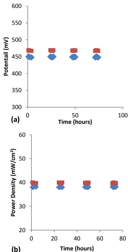
**Figure 6.** DMFC,  $\blacklozenge$  Nafion 117,  $\blacksquare$  0.5% loading (a) potential and (b) power density variation during 100 hour operation using a single cell DMFC operating at 70°C, 1 M methanol feed, and at a current of 80 mA cm<sup>-2</sup>.
