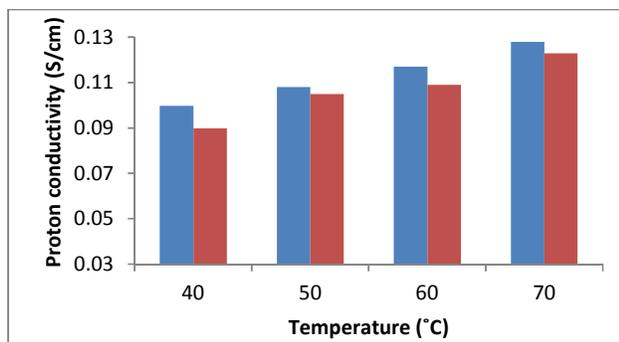
**Figure 9.** ■ Nafion 117, ■ 0.5% loading. Proton conductivity of MEAs determined using impedance spectroscopy at OCV with a 1M methanol feed at a range of operating temperatures and mordenite loading in the barrier layer.
