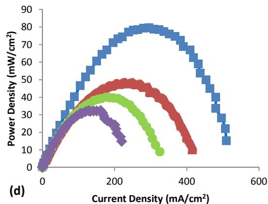
**Figure 1.** Experimental results showing DMFC performance for a standard Nafion 117 MEA. ■ 70°C, ▲ 60°C, ● 50°C, ◆ 40°C. (a,b) compared with an MEA incorporating a functionalised mordenite composite layer with a loading of 0.5% mordenite (c,d). A 1M methanol feed and operating temperatures between 40°C and 70°C were used. (a and c) Polarization curves (b and d) Power Density curves.
