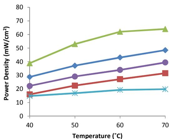
**Figure 3.** DMFC peak power densities with a 2 M methanol feed. ◆ Nafion 117, ■ 0.25% loading, ▲ 0.5% loading, ● 0.75% loading, × 1% loading using a standard MEA and MEAs featuring a mordenite composite layer with a range of mordenite loadings (from 0.25 % to 1.0 %).
