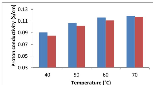
**Figure 10.** ■ Nafion 117, ■ 0.5% loading. Proton conductivity of MEAs determined using impedance spectroscopy at OCV with a 2M methanol feed at a range of operating temperatures and mordenite loading in the barrier layer.
