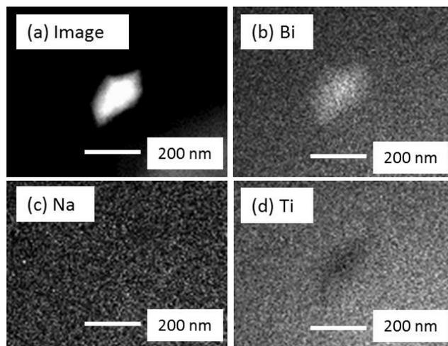
**Figure 3.** (a) HAADF-STEM (Z-contrast) images for  $x = 0.01$  and EDX mapping results of the same area for (b) Bi-mapping, (c) Na-mapping and (d) Ti-mapping.
