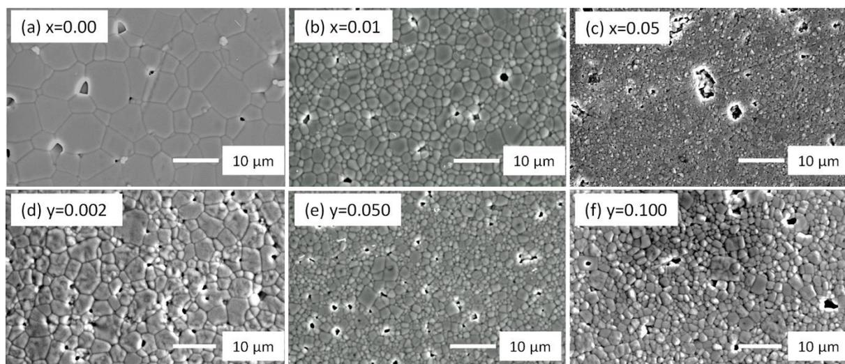
Figure 4. SEM micrographs, (a) to (c) for selected  $\text{Na}_{0.50}\text{Bi}_{0.50+x}\text{TiO}_{3-3x/2}$  and (d) to (f) for selected  $\text{Na}_{0.50}\text{Bi}_{0.50}\text{Ti}_{1-y}\text{Nb}_y\text{O}_{3-y/2}$  ceramics.
