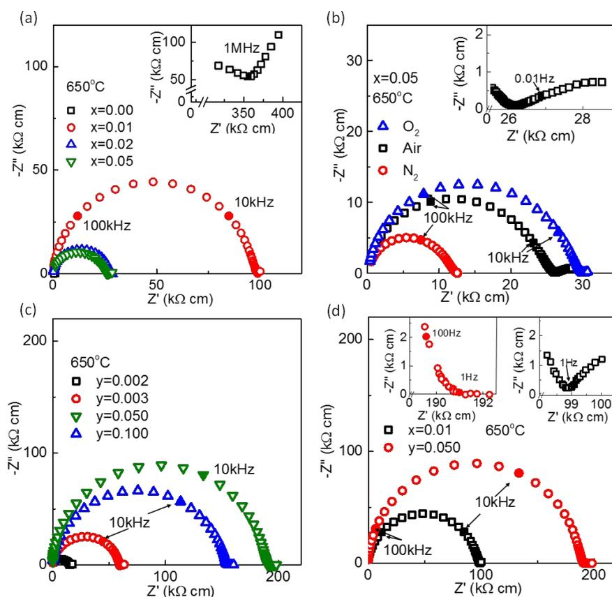
Figure 5.  $Z^*$  plots of selected (a)  $\text{Na}_{0.50}\text{Bi}_{0.50+x}\text{TiO}_{3-3x/2}$  ceramics, (b)  $x = 0.05$ , Type II ceramic, (c) selected  $\text{Na}_{0.50}\text{Bi}_{0.50}\text{Ti}_{1-y}\text{Nb}_y\text{O}_{3-y/2}$  ceramics and (d)  $x = 0.01$  and  $y = 0.050$  Type III ceramics. All data were obtained at  $650^\circ\text{C}$
