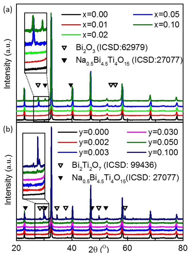
**Figure 1.** Room temperature X-ray powder diffraction data for (a)  $\text{Na}_{0.50}\text{Bi}_{0.50+x}\text{TiO}_{3+3x/2}$  and (b)  $\text{Na}_{0.50}\text{Bi}_{0.50}\text{Ti}_{1-y}\text{Nb}_y\text{O}_{3+y/2}$  series of crushed ceramics.
