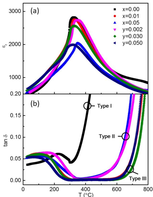
**Figure 7.** (a)  $\epsilon_r$  and (b)  $\tan \delta$  (both at 1 MHz) versus temperature for selected  $\text{Na}_{0.50}\text{Bi}_{0.50+x}\text{TiO}_{3+3x/2}$  and  $\text{Na}_{0.50}\text{Bi}_{0.50}\text{Ti}_{1-y}\text{Nb}_y\text{O}_{3+y/2}$  ceramics.
