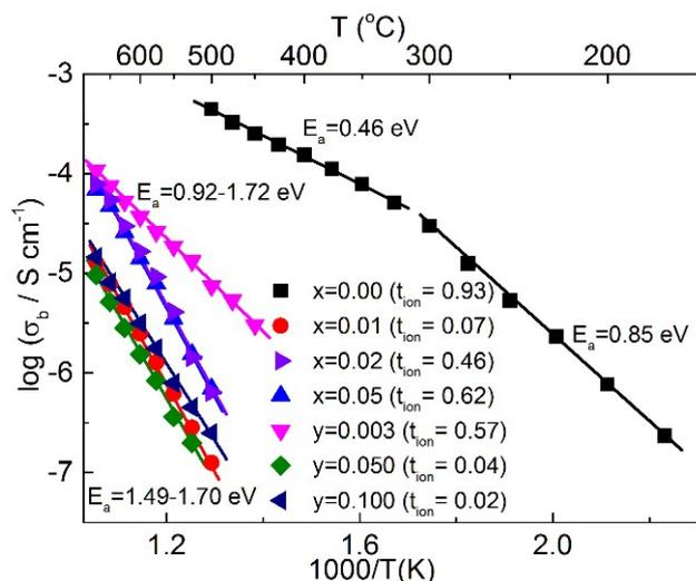
**Figure 6.** Arrhenius plot of bulk conductivity,  $\sigma_b$ , versus reciprocal temperature for selected  $\text{Na}_{0.50}\text{Bi}_{0.50+x}\text{TiO}_{3+3x/2}$  and  $\text{Na}_{0.50}\text{Bi}_{0.50}\text{Ti}_{1-y}\text{Nb}_y\text{O}_{3+y/2}$  ceramics. Activation energy,  $E_a$ , values for  $\sigma_b$  and  $t_{\text{ion}}$  values at 600 °C are included.
