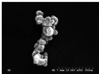
Fig. 6 SEM image vesicles of 2 (0.075 μM solution sonicated for 5 minutes).
