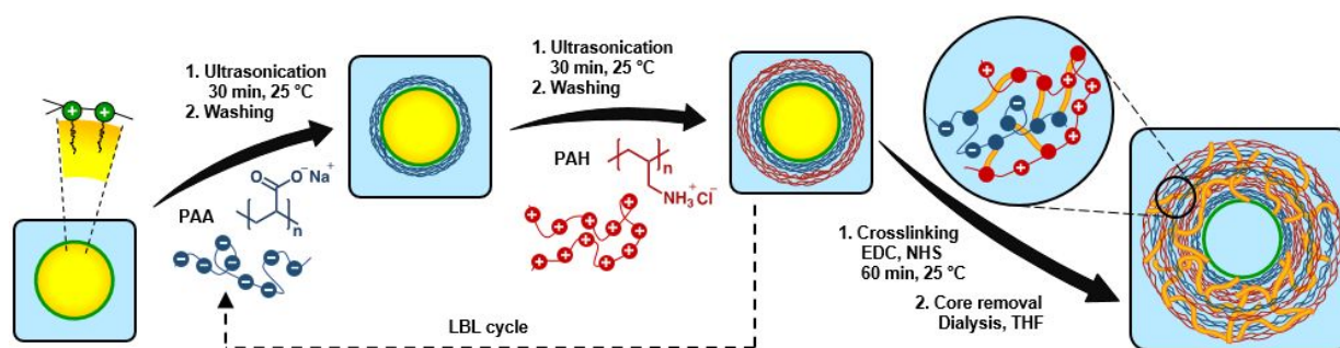
Scheme 1. LBL synthesis of crosslinked PEM NCs using crystallized miniemulsion NPs with covalently-stabilized surfactant layers as substrate.
