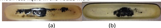
Figure 9. Light micrographs of (a) Bi-2212 (890 °C/2h) and (b) Yb123 pellets (915 °C/2h) after melting and rapid cooling to room temperature in flowing O 2 .
