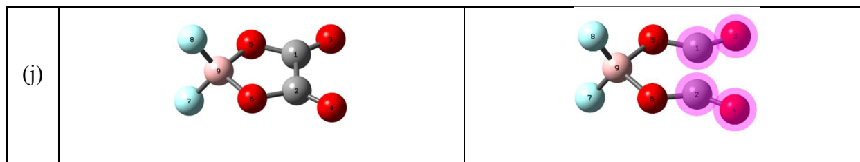
Figure 2. Optimized Geometries of Isolated Solvents, Anions, and Additives both in the Initial and Oxidized States in the Solution Phase. White, peach, grey, blue, red, cyan, and yellow colors represent H, B, C, N, O, F, and S atoms, respectively. The atoms with significant positive spin densities by oxidation are highlighted in magenta.
