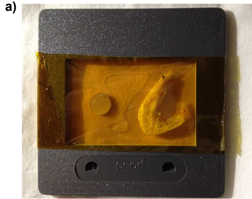
Figure 1. Sample preparation for SR- \mu XRF analysis at the CHESS F3 station: (a) shrimp and CRM pellet mounted on 24x36 mm slide using Kapton ® tape and (b) a powdered As compound contained within a teflon washer and secured with Kapton ® tape.
