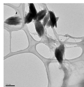
Fig. 8. TEM of the loosely bound deposits that are formed around the anode, which are easily dislodged and re-suspended when electrodes were taken out of the bath and subsequently deposited on the lacy carbon TEM grid. Scale bar = 200 nm.
