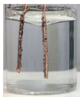
Fig. 1. Photographs of raw SWCNTs after 102 seconds electrolysis in DI water. The left electrode is the anode while the right electrode is the cathode.
