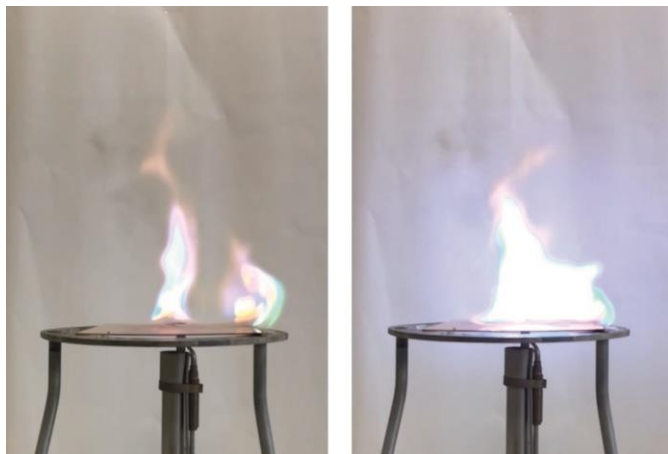
Figure 17 Moment of deflagration of compound 8 during the hot plate test shown as a sequence.
