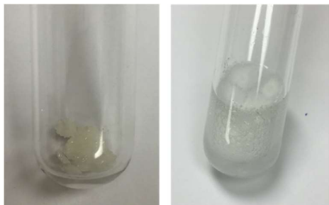
Figure 3. Left: Crystals of the desipramine-CO 2 ammonium carbamate salt. Right: Same salt upon addition of water at pH = 2.0, within the normal gastric pH range. The evolution of CO 2 is apparent. Subsequent evaporation of water and analysis by 1 H- and 13 C-NMR revealed the re-formation of desipramine hydrochloride, the form of the drug currently in clinical use.
