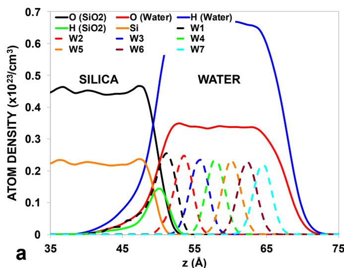
Figure 2. (a) Density profiles of atoms in the glass and water;  $W_i$  indicate location of the O atoms in water as a function of water ‘layer’ based on H-bonding (see text). (b) side view of system with Si atoms in blue, SiO bonds in grey, and water OH bonds in cyan; (c) SiO bonds at  $z > 49$  Å and  $z < 38$  Å and water oxygen at  $z < 49$  Å shown as cyan spheres. (c) shows water penetrating 11 Å below outer Si atoms at 300K.
