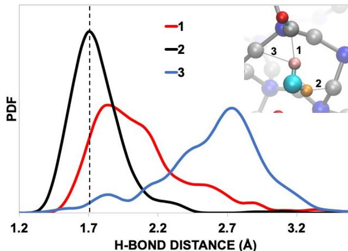
Figure 10. Labeled H-bond lengths for H<sub>2</sub>O molecule shown in inset and figure 9 showing asymmetric H-bonds. H-bond labeled 2 shorter than normal H-bond in water (1.70 Å peak max) vs. 1.8 Å for water).
