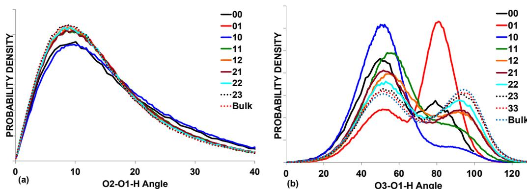
Figure 4. Bond angles for O2-O1-H in (a) and O3-O1-H in (b) and provides location of proton's second acceptory O (see text). O<sub>i</sub> given in figure 3a inset. Legend as in figure 3.
