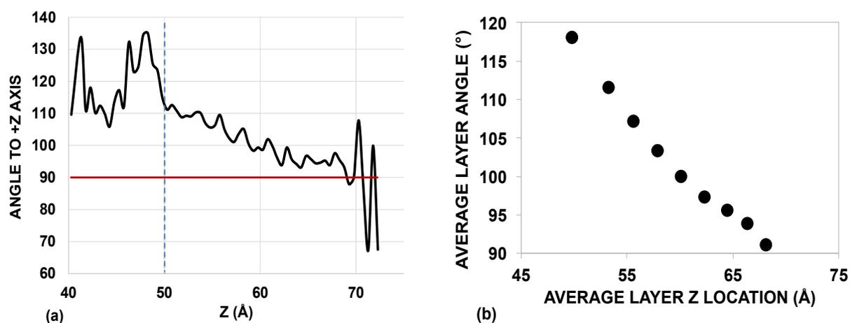
Figure 5. (a) Dipole moment orientation of water molecules related to the +Z axis direction. Vertical dashed line indicates approximate location of glass surface. (b) Average angle of the dipole moment relative to the +Z axis for each water 'layer'.
