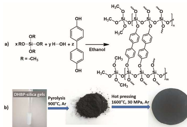
Fig. 2. Sol-gel synthesis of orthosilicate-based single-source precursors containing large, aromatic substituents (a); their ceramization at 900^\circ\text{C} and uniaxial hot pressing at 1600^\circ\text{C} in Ar atmosphere to produce monolithic ceramic samples (b).
