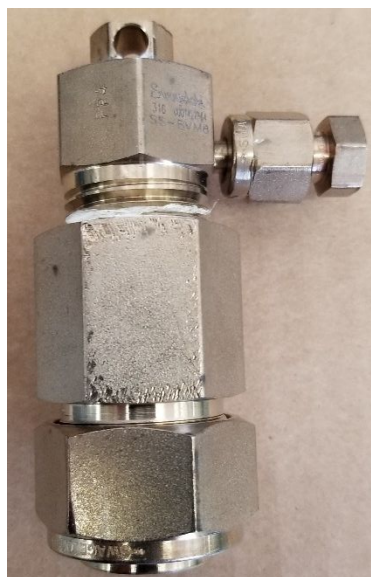
Figure 1. One of the assembled Swagelok reactors used for all SCM-DHDO reactions. The reactors are opened via the bottom \frac{3}{4} " Swagelok plug while purging and gas sampling is done through the \frac{1}{2} " NPT bleed valve on the top.
