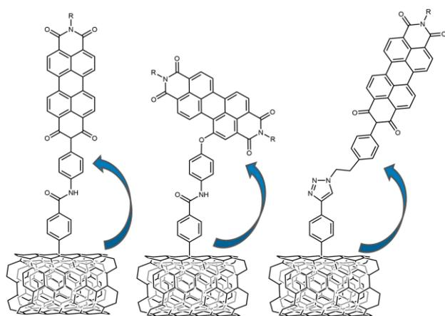
**Figure 8.** Covalent grafting of PDIs onto the DWCNT external wall via amide bond formation and 'click' chemistry.
