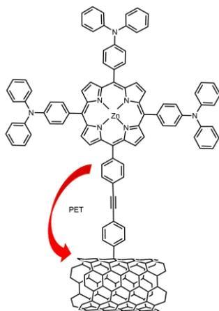
**Figure 5.** D-A hybrid system involving an electron donor ZnPor and SWCNT obtained via a two-step reaction (Diazonium salt chemistry + Sonogashira cross coupling).
