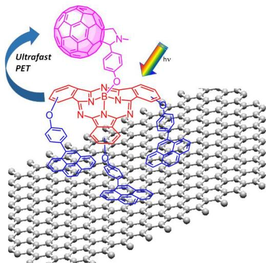
**Figure 17.** Structure of the subphthalocyanine-fullerene tethered with three pyrene units, (Pyr)<sub>3</sub>SubPc-C<sub>60</sub> donor-acceptor conjugate, interacting with graphene.
