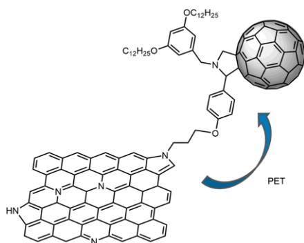
**Figure 12.** Schematic representation of the electron-transfer process observed in an NG- $\text{C}_{60}$  hybrid where NG behaves as the electron-donor.
