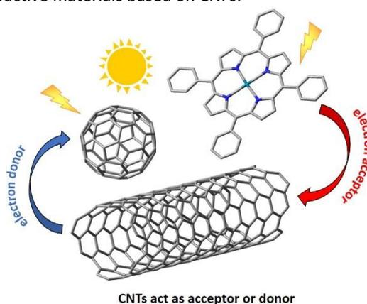
**Figure 1.** Bidirectional charge transfer behaviour shown by carbon nanotubes under light excitation when they are interfaced with different types of electroactive counterparts.
