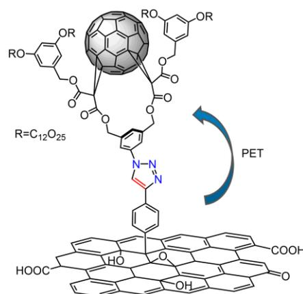
**Figure 11.** Schematic representation of the electron-transfer process observed in a GO- $C_{60}$  hybrid where GO behaves as the electron-donor.
