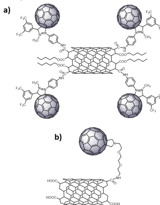
**Figure 6.** Hybrid structures involving SWCNTs and different electron-acceptor moieties: a) pyrazolinofullerene derivatives and b) pyrrolidinofullerene derivatives.
