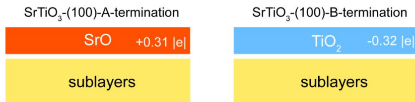
Fig. 6. Charge of surface layers on SrTiO 3 (100) for A-termination and B-termination. The surface-layer charge is determined by the sum of the Bader charges of all the atoms in the top layer of the surface before Pt 1 adsorption (Table 1).
