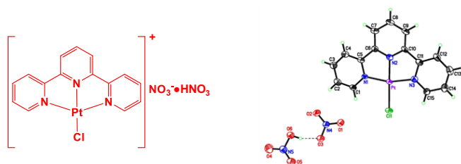
Fig. 1. (left) Molecular structure of the formula unit of the salt [\text{Pt}(\text{tpy})\text{Cl}]\text{NO}_3\cdot\text{HNO}_3 ( 1\cdot\text{NO}_3\cdot\text{HNO}_3 ). (right) ORTEP of 1\cdot\text{NO}_3\cdot\text{HNO}_3 .
