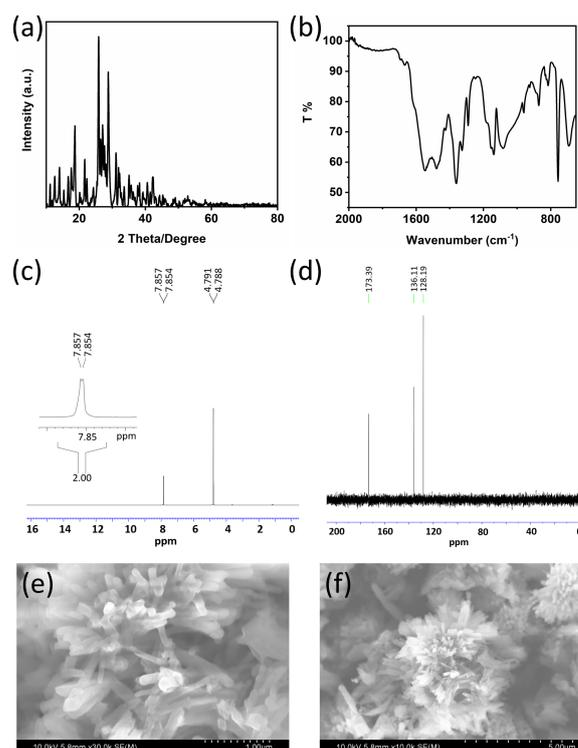
**Fig. 1.** Material characterizations for  $\text{Na}_4\text{C}_{10}\text{H}_2\text{O}_8$ . (a) XRD pattern, (b) FTIR spectrum, (c)  $^1\text{H}$  NMR spectrum, and (d)  $^{13}\text{C}$  NMR spectrum. SEM images with scale bars of (e)  $1\ \mu\text{m}$  and (f)  $5\ \mu\text{m}$ .
