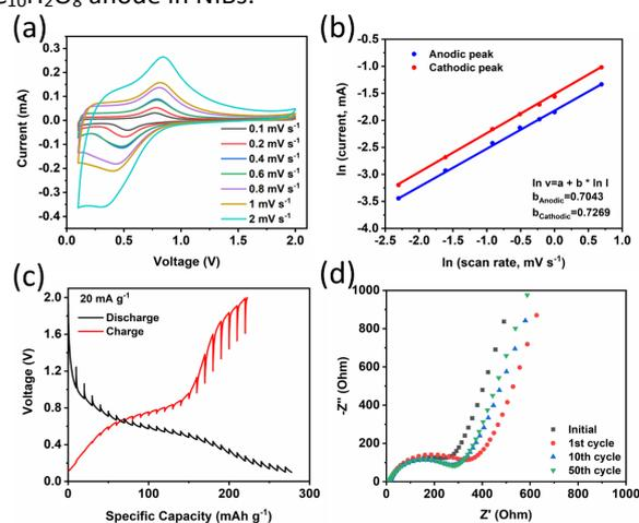
**Fig. 3.** Reaction kinetics of  $\text{Na}_4\text{C}_{10}\text{H}_2\text{O}_8$  in NIBs. (a) Cyclic voltammograms at various scan rates; (b) The  $\ln$  relationship of peak current and scan rate; (c) Potential response during GITT measurements; (d) Impedance analysis before and after charge/discharge.
