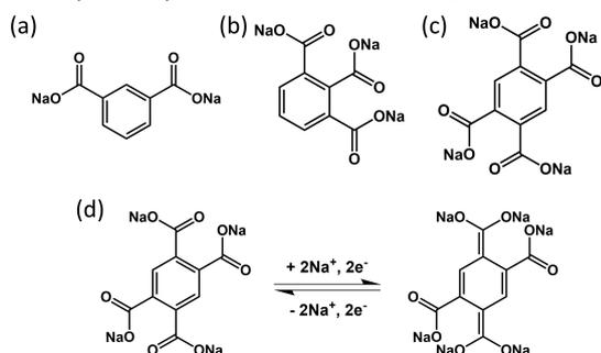
**Scheme 1.** The molecular structure of three sodium carboxylates: (a)  $\text{Na}_2\text{C}_8\text{H}_4\text{O}_4$ , (b)  $\text{Na}_3\text{C}_9\text{H}_3\text{O}_6$ , and (c)  $\text{Na}_4\text{C}_{10}\text{H}_2\text{O}_8$ ; (d) The sodiation/de-sodiation mechanism of  $\text{Na}_4\text{C}_{10}\text{H}_2\text{O}_8$ .
