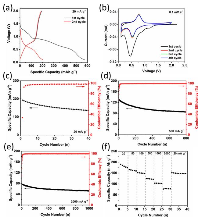
**Fig. 2.** Electrochemical performance of  $\text{Na}_4\text{C}_{10}\text{H}_2\text{O}_8$  in NIBs. (a) Galvanostatic charge-discharge curves; (b) Cyclic voltammograms at  $0.1 \text{ mV s}^{-1}$ ; De-sodiation capacity and Coulombic efficiency versus cycle number at the current density of (c)  $20 \text{ mA g}^{-1}$ , (d)  $500 \text{ mA g}^{-1}$ , (e)  $2000 \text{ mA g}^{-1}$ ; (f) Rate performance at various current densities.
