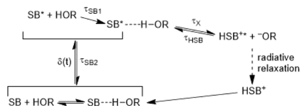
Fig. 5 Kinetic model for the ESPT reaction between FRO-SB and the alcohol solvent ROH.
