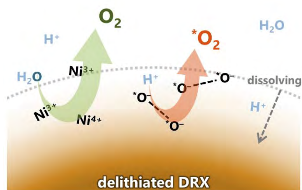
Fig. 3 Illustration of decoupled \text{O}_2 -release reactions during the ex-situ acid titration of NTMF. Gray dotted curve outlines the acid-particle interface before dissolution. Star symbols indicate partial ^{18}\text{O} enrichment. Dissolved oxygen anions with formal valence of -1 ( \text{O}^- ) are displayed to represent all possible lattice oxidized oxygen species (ESI† Note S2). Other dissolved species, such as \text{Li}^+ and \text{F}^- , not participating in \text{O}_2 -release reactions are not shown for clarity.
