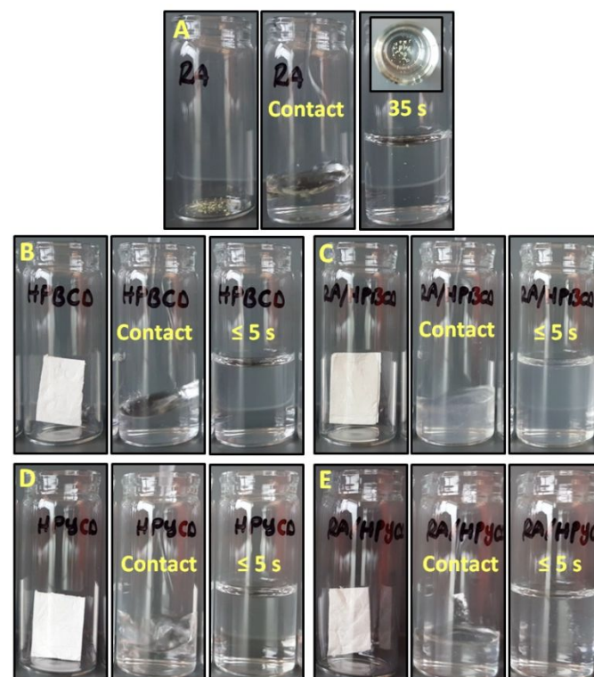
Fig. 7 The dissolution behaviour of samples in water. (A) Vitamin-A acetate powder, (B) HP \beta CD-NW, (C) Vitamin-A acetate/HP \beta CD-NW, (D) HP \gamma CD-NW and (E) Vitamin-A acetate/HP \gamma CD-NW. These pictures were captured from Video S1.
