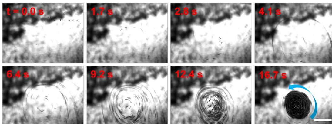
**Fig. 3** Frames depicting the particle concentration effect in the acoustic vortex ( $20\ \mu\text{m}$  particles) generated in the flexural-wave-based acoustofluidic device. Using a  $5.3\ \text{kHz}$  signal applied to both transducers, a rotating mass of particles has formed on the surface of the liquid in the device within 17 seconds. Scale bar:  $500\ \mu\text{m}$ .
