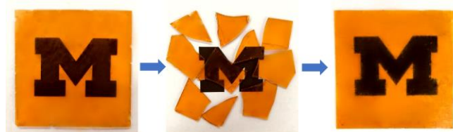
Fig. 14 The initial TE-BMIO-EG thermoset film, the broken film, and the remolded film. The logo beneath the film demonstrates the transparency of the film.
