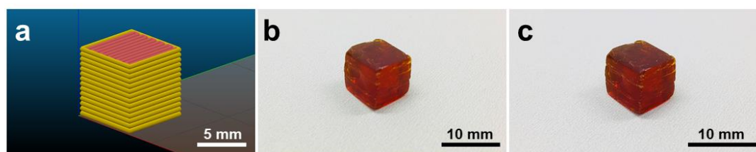
Fig. 7 (a) The original design of a 7 mm × 7 mm × 7 mm cube. (b) The image of the as-printed cube. (c) The printed cube after curing overnight.
