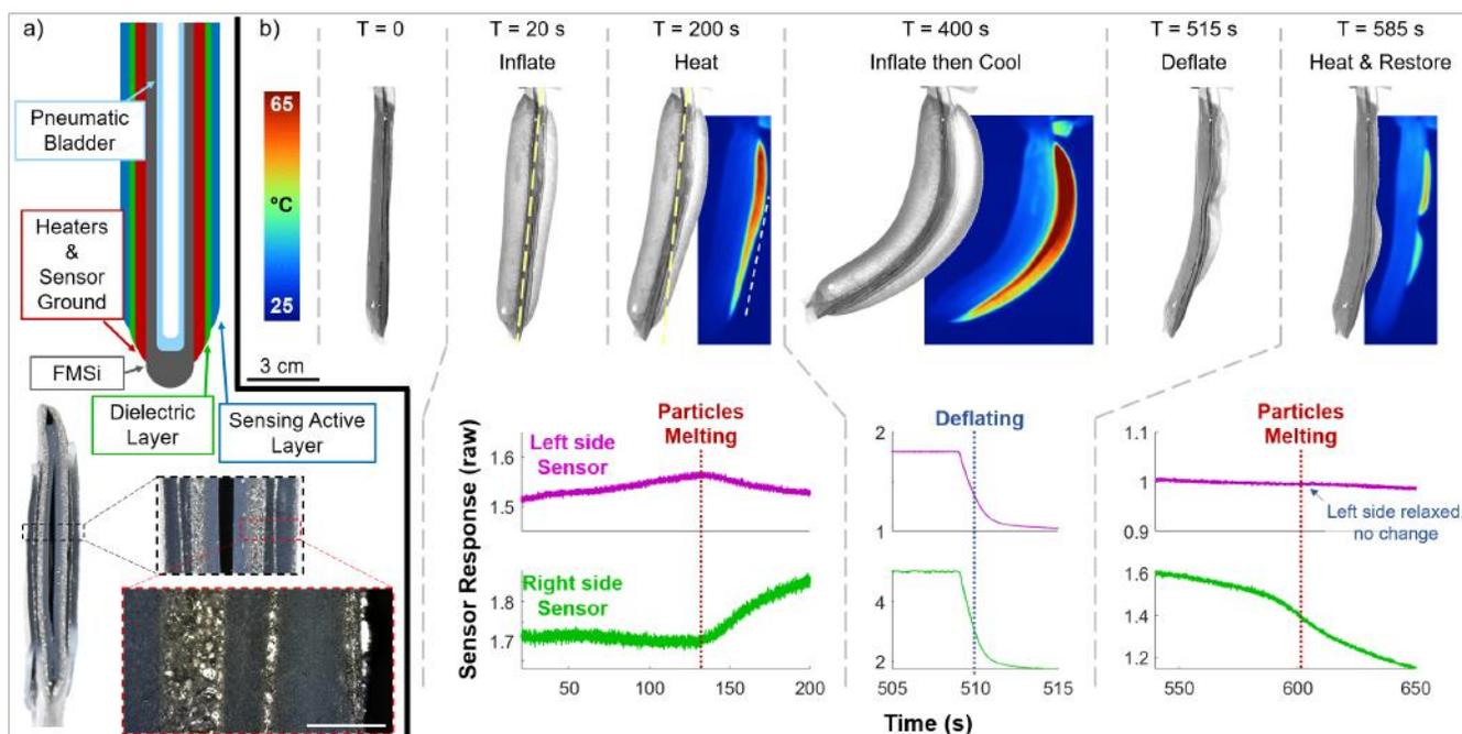
Fig. 8 MPC silicone applied as a heater and a sensor on a stiffness-changing pneumatic bladder. a) Schematics and photographs of the cross section of the pneumatic bladder. Inset scalebar is 1 mm. Silicone glue layers are not shown in the schematic unless they serve an additional functional purpose b) Visible light and IR photographs of the sensorized bladder at various times, along with graphs of the raw sensor response as the system undergoes both temperature and pressure changes.
