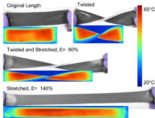
Fig. 1 An activated  $4 \times 16$  cm sample of the MPC being simultaneously twisted and stretched, while maintaining a consistent, uniform Joule heating profile. The sample is fully encapsulated in silicone.
