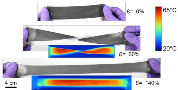
A thin, stretchable (200% linear strain), multiphase (solid-liquid) silicone composite with uniform electrical conductivity, for Joule heating and high-deformation sensing.
