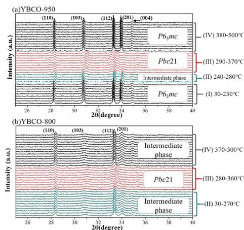
Fig. 3. In-situ high temperature XRD results of  $\text{YBaCo}_4\text{O}_{7+\delta}$  in  $2\theta$  of 25–40°. (a) 950 °C sample from 30 to 500 °C heating at air atmosphere including four areas. (b) 800 °C sample from 30 to 500 °C heating in the air atmosphere including three areas.
