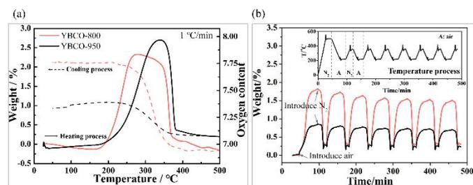
Fig. 2. (a) TG curves of  $\text{YBaCo}_4\text{O}_{7+\delta}$  in the air atmosphere from 30 °C to 500 °C with heating/cooling rates of 1 °C/min for 800 and 950 °C samples. (b) TG curves of  $\text{YBaCo}_4\text{O}_{7+\delta}$  measured by TSA processes during swing between 220 and 360 °C.  $\text{N}_2$  is the reducing gas, air is the oxidizing gas. (insert picture: temperature process)
