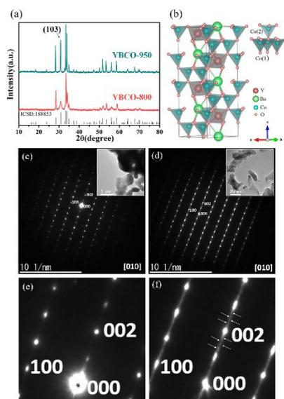
Fig. 1 (a) XRD patterns of  $\text{YBaCo}_4\text{O}_{7+\delta}$  synthesized at different calcination temperatures. (b) The standard model structure of  $\text{YBaCo}_4\text{O}_7$ . The [010]-incidence ED patterns of (c) 950 °C sample and (d) 800 °C sample. Enlarged ED patterns of (e) 950 °C sample and (f) 800 °C sample.
