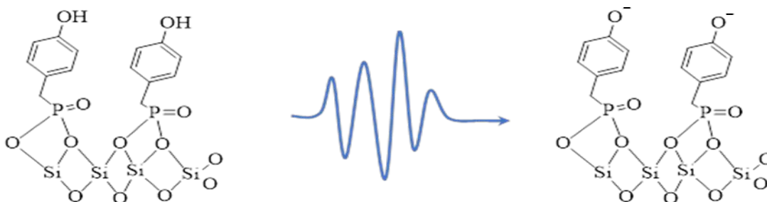
Figure 1: Schematic representation of phosphonated phenol molecules bound to a silicon dioxide surface where the hydroxyl group undergoes optically induced deprotonation.
