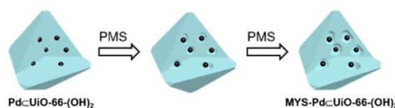
Figure 36. Schematic illustration of the oxidative linker cleaving process used to install Pd NPs in a multiple core-shell fashion. Adapted with permission from ref. 252. Copyright 2019 American Chemical Society.
